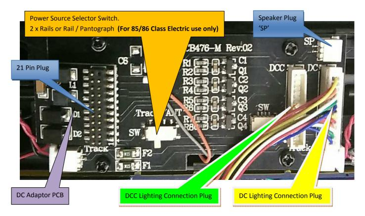
• In order to adjust the running qualities of your model for your personal preference, reference to suggested settings in the form of a quick start guide is available in the following notes. Alternatively for full decoder adjustment details refer to the ESU Loksound V5 Decoder Manual and Full Throttle Description available at the following links:
