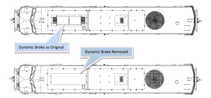
With the dynamic brake removed, these locomotives lost all dynamic brake functionality including engine rpm's increasing and the grid fans no longer sounding.
